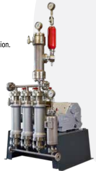
FELUWA MULTISAFE® double hose-diaphragm pump Example application: TG 135 – 3 DS 100 Triplex, single-acting pump: 24 to 47 m 3 /h at 70 bar and 100 °C Medium: aggressive and abrasive chemical catalyst Media-contacting components made of 1.4410 (Super Duplex) and hose-diaphragms of EPDM
